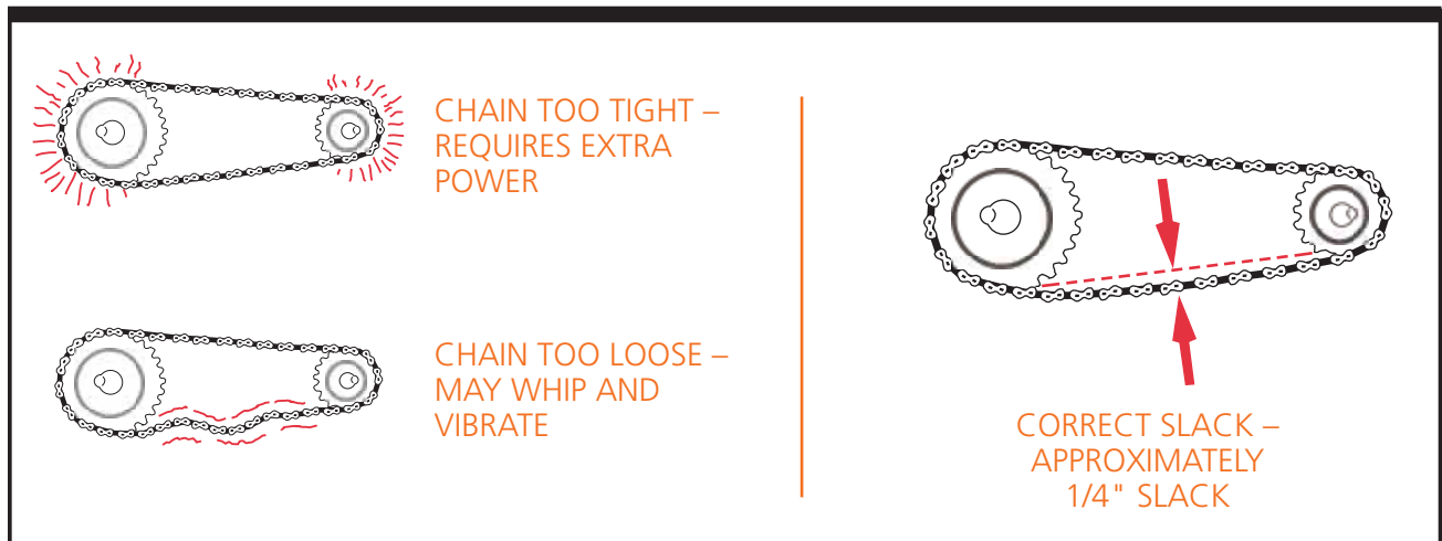
Figure 4-1. Chain Tensions
