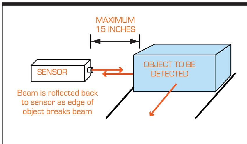
Figure 4-6. Setup for Product Sensor
