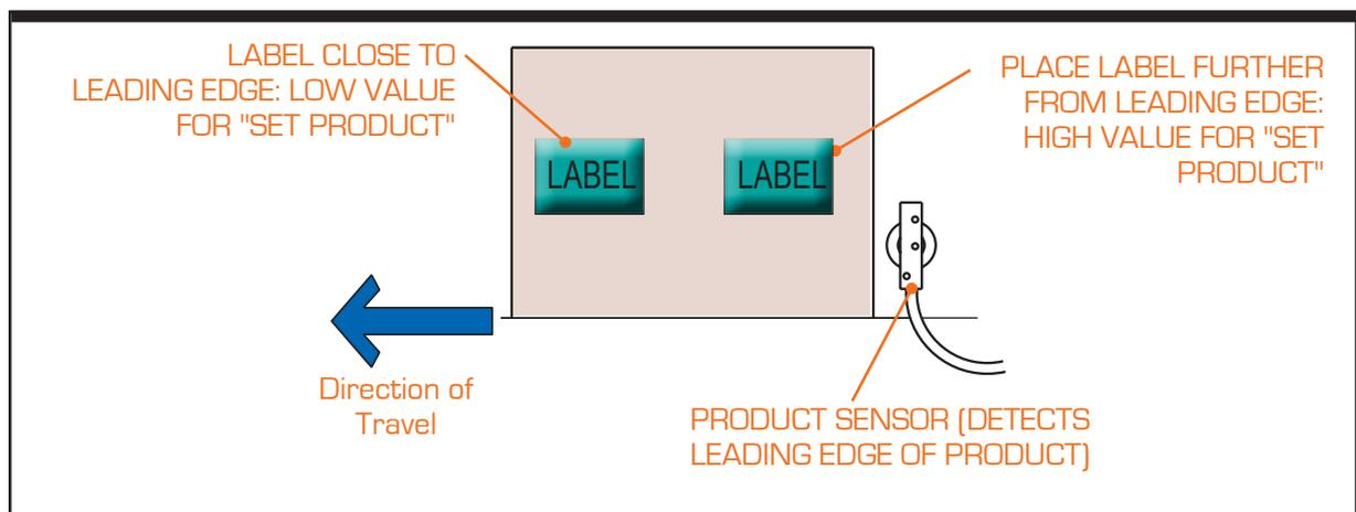
Figure 5-14. Fine Tuning Label Placement
