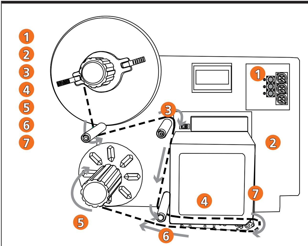
Figure 4-1. Web Path (Left Hand Labeler Shown)
