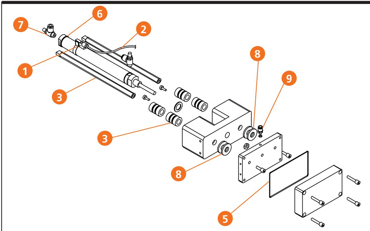
Figure 8-3. L3500PA Tamp Module Parts Callouts
