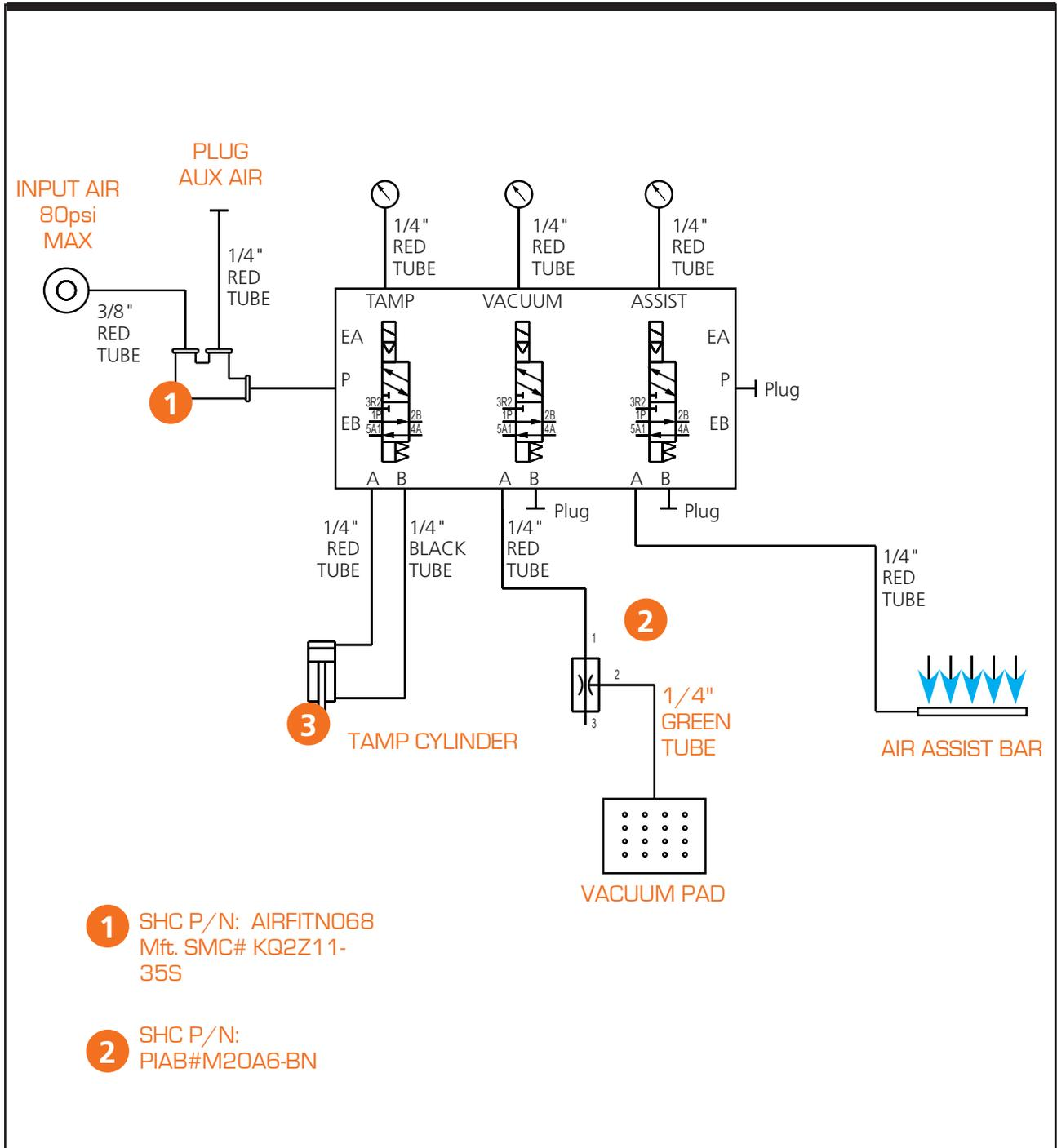
Figure 10-1. Pneumatic Schematics
