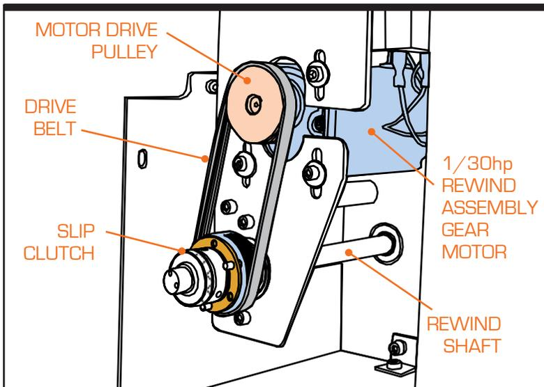
Figure 4-4. Clutch Assembly for Rewind Assembly (Rear of Labeler)
