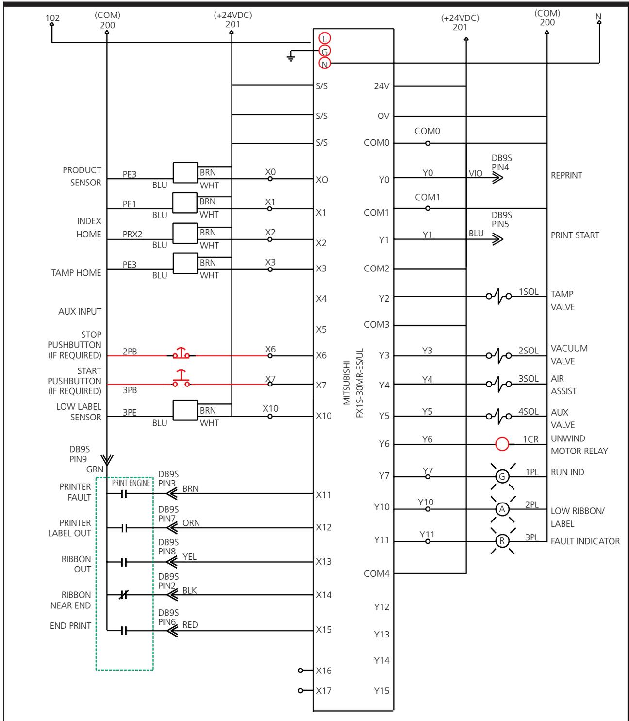
Figure 10-2. Labeler System Power/Control Wiring (Part 2)
