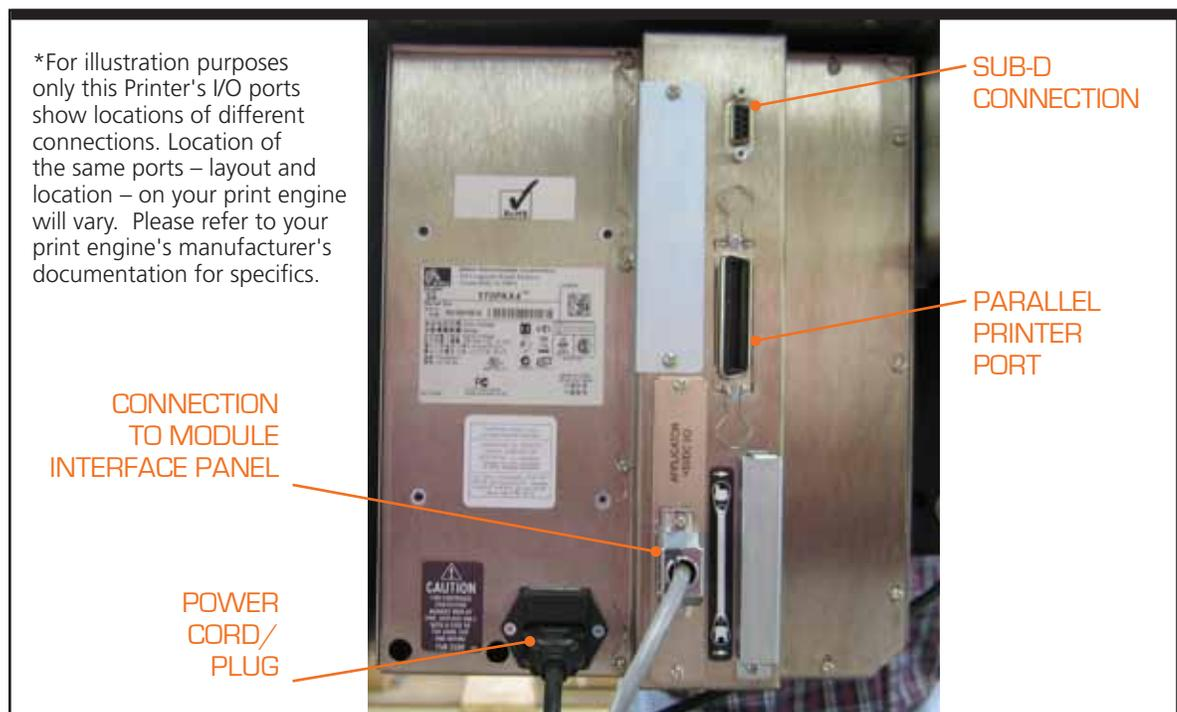
Figure 3-6. Printer I/O Ports (Example)
