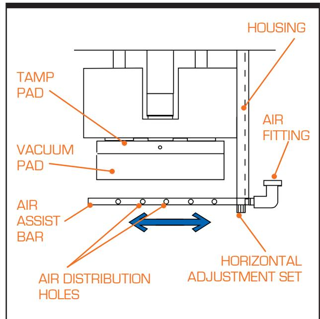
Figure 5-7. Air Assist Bar
