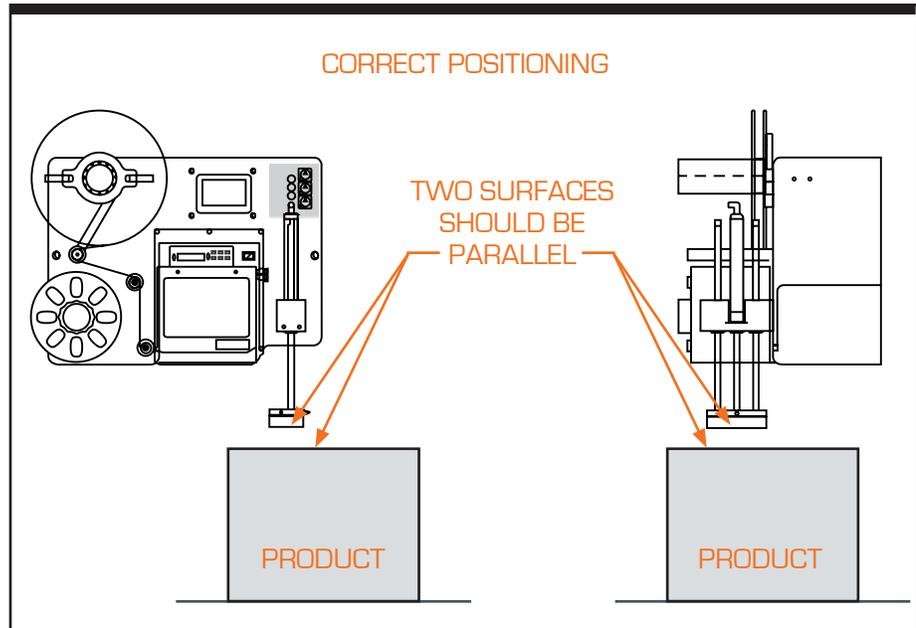
Figure 3-1. Correct Positioning of Labeler
