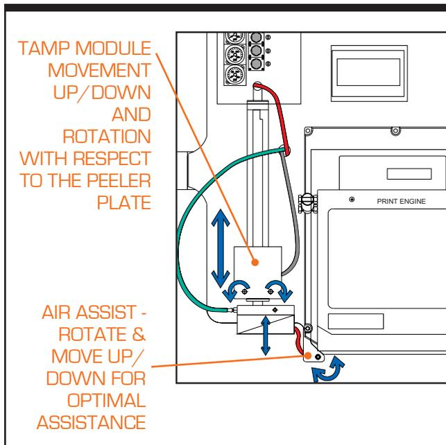
Figure 5-6. Tamp Adjustments When Feeding A Label
