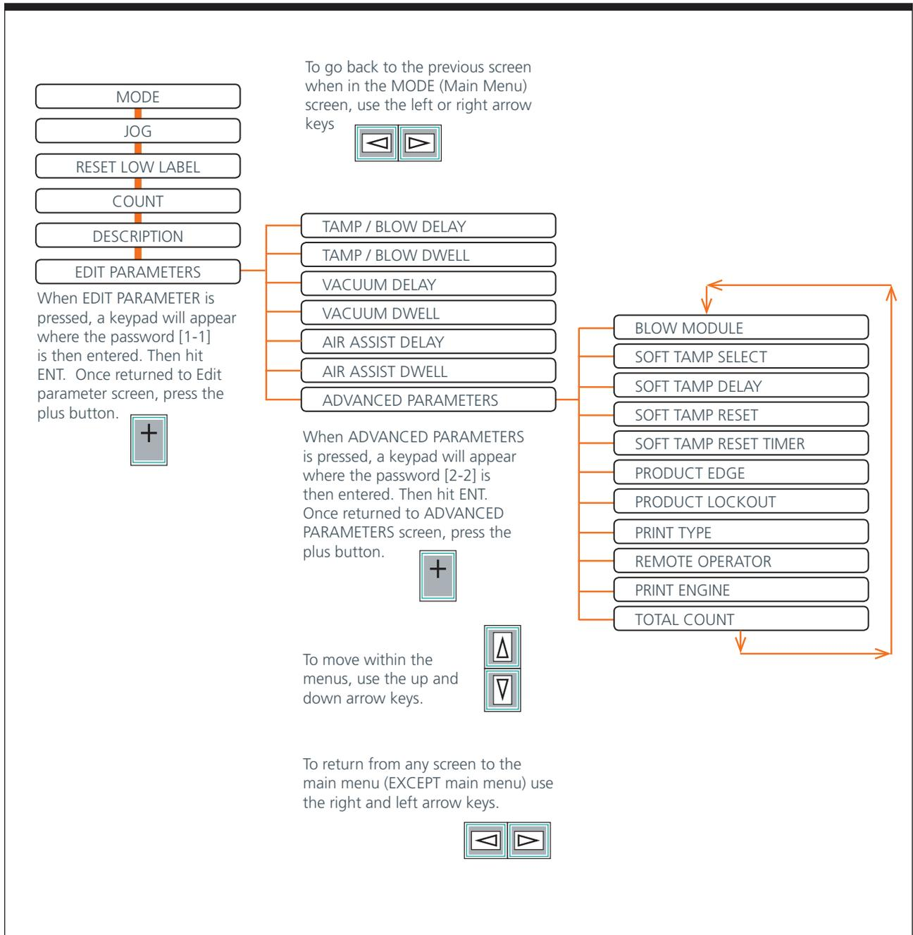
Figure 6-1. Mapping of the Operator Interface
