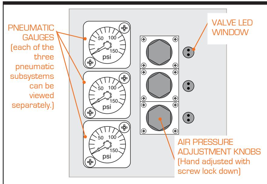
Figure 3-8. Pneumatic Valve Pack (Front View)
