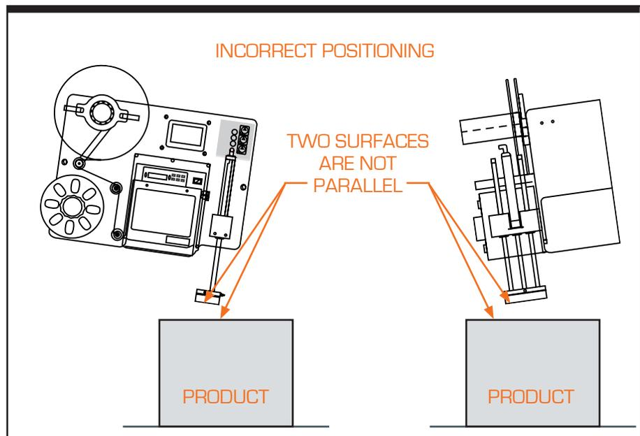
Figure 3-2. Incorrect Positioning of Labeler
