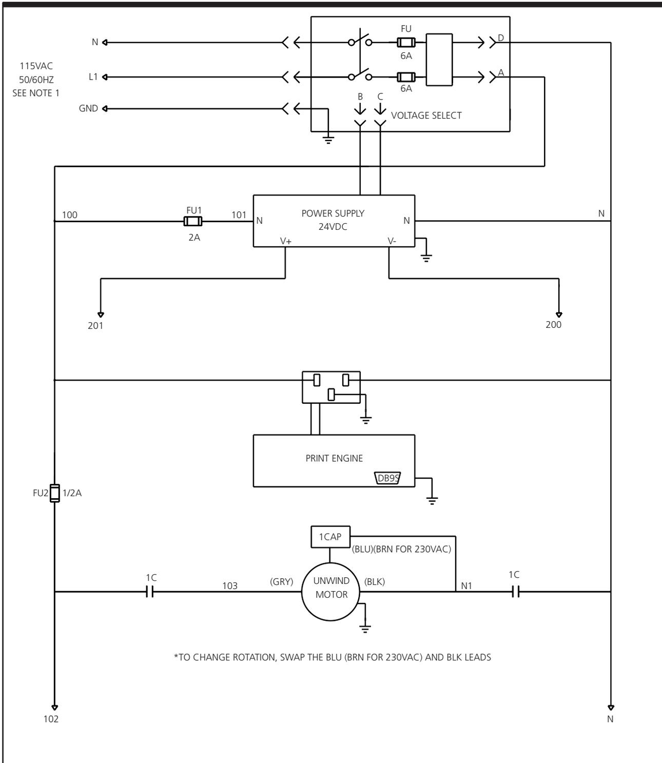
Figure 10-2. Labeler System Power/Control Wiring (Part 1)
