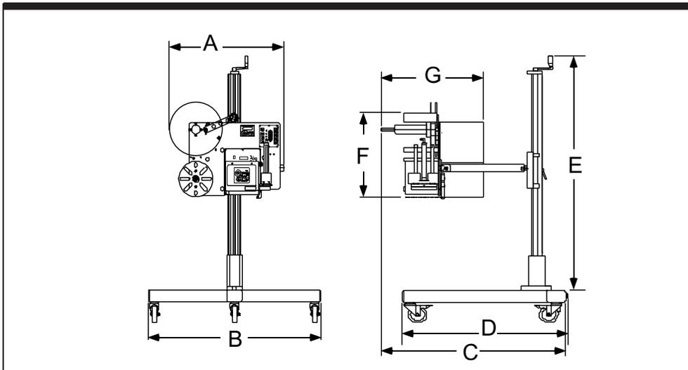
Figure 1-1. L3500PA Side and Front Views with Dimensions
