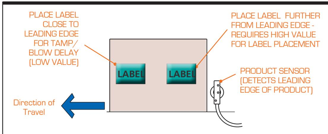
Figure 5-8. Fine Tuning Label Placement
